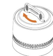
1) Activate the smoke alarm by pushing the mounting plate and turning it clockwise at the same time. The smoke alarm is activated and ready to be installed when you feel clicks. you may also hear an alarm sound if the test button gets pressed during activation.
