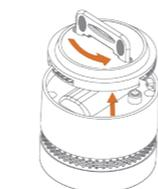
1) Remove the mounting plate of the smoke alarm by turning it counterclockwise and lifting it away.
