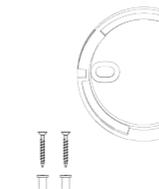
2) To achieve the correct smoke alarm positioning, then mark drill holes for the screw anchors. install the mounting plate of the smoke alarm tightly to the ceiling with the screws.
