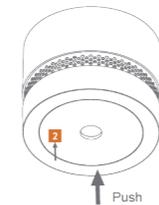
4) Attach the smoke alarm by pressing it firmly against the ceiling for approximately 60 seconds. You may also hear an alarm sound if the test button gets pressed during installation.
