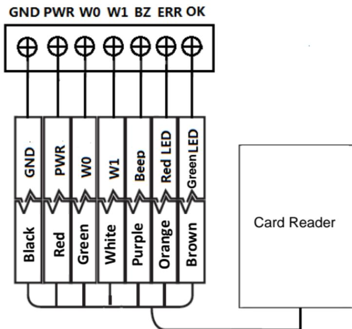
Figure 3-5 Wiring for Wiegand Communication Mode
