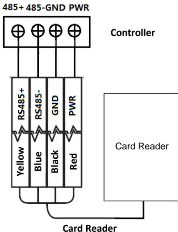
Figure 3-4 Wiring for RS-485 Communication Mode
