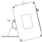
Figure 2-4 Rail-Mounted Installation
