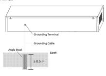
Figure 3-2 Grounding with Angle Steel
