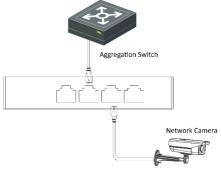
Figure 3-3 RJ45 Port Connection
