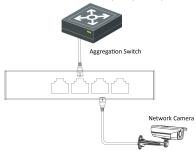
Figure 3-3 RJ45 Port Connection
