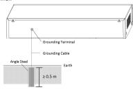
Figure 3-2 Grounding with Angle Steel
