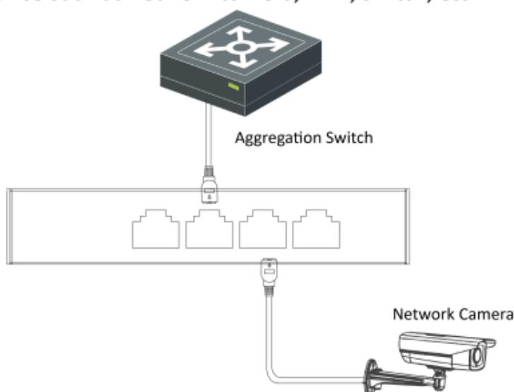
Figure 3-3 RJ45 Port Connection
