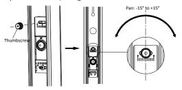
Figure 2-15 Install Thumbscrew and Adjust Panning Position
