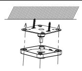
Figure 2-24 Hood the Bracket Cover
