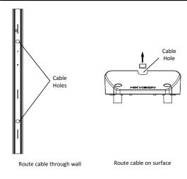
Figure 2-13 Plan Cable Routing
