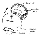
Figure 2-32 Install the Camera and Bracket Cover
