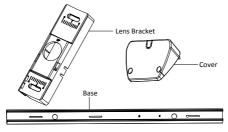
Figure 2-9 Pole-Shaped Bracket Component
