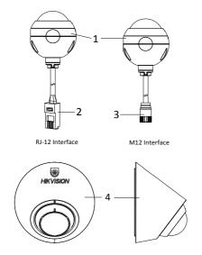
Figure 1-9 Ball-Shaped Sensor Unit and Included Bracket
