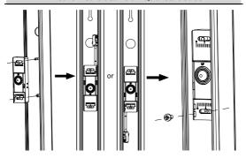
Figure 2-14 Install and Secure Lens Bracket
