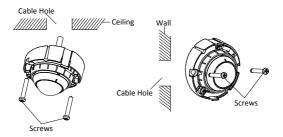
Figure 2-37 Fix the Camera and Mounting Base to Wall or Ceiling
