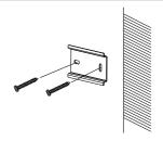
Figure 2-1 Secure the Mounting Rail
