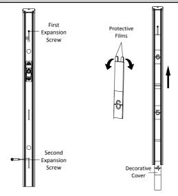
Figure 2-17 Secure Base on Wall
