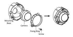
Figure 2-36 Fix the Camera to Mounting Base
