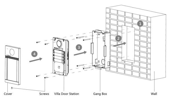
Figure 3-9 Flush Mounting without Protective Shield
