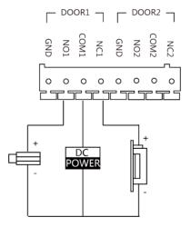
Figure 2-2 Door Lock Wiring
