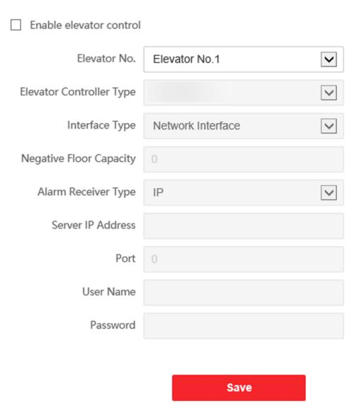
**Figure 5-24 Elevator Control**
