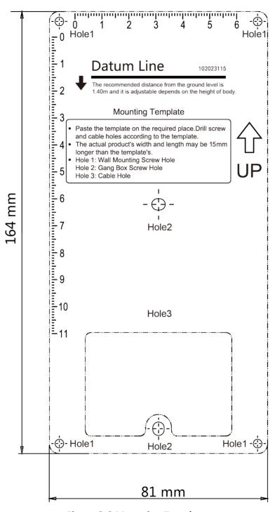
**Figure 3-8 Mounting Template**
