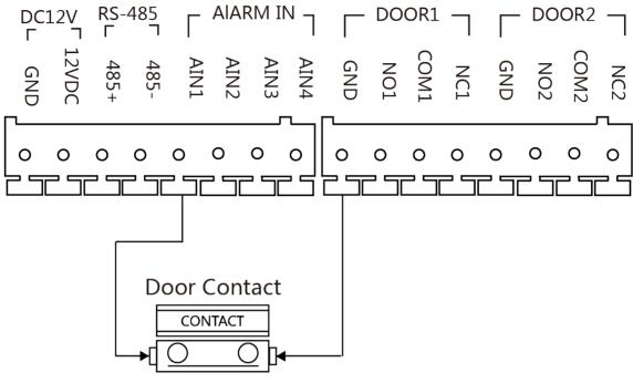
**Figure 2-3 Door Contact Wiring**
