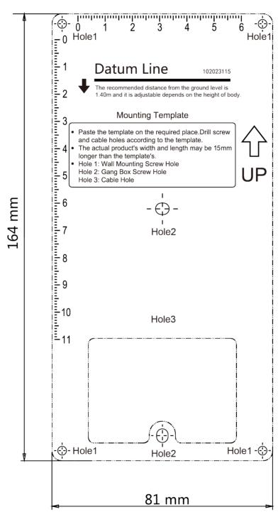
**Figure 3-2 Mounting Template**
