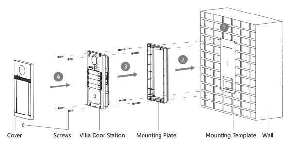
Figure 3-5 Surface Mounting without Protective Shield
